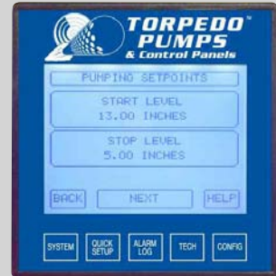
Pump on/off level setup
