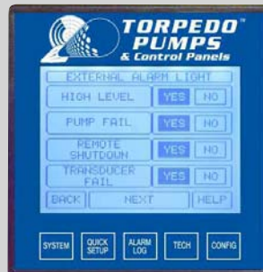
Alarm condition setup
